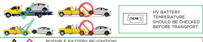
POSSIBLE BATTERY RE-IGNITION! AFTER A FIRE INCIDENT, STORE OUTSIDE AT A SAFE DISTANCE (AT LEAST 50 FT/15 M) FROM OTHER VEHICLES AND STRUCTURES!
